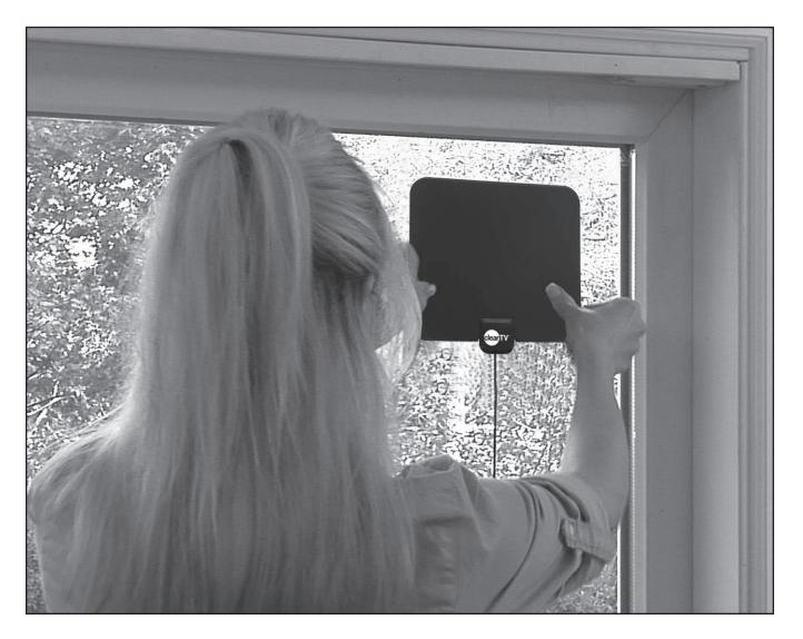
**Step 2B** — MOUNTING ANTENNA TO WINDOW
